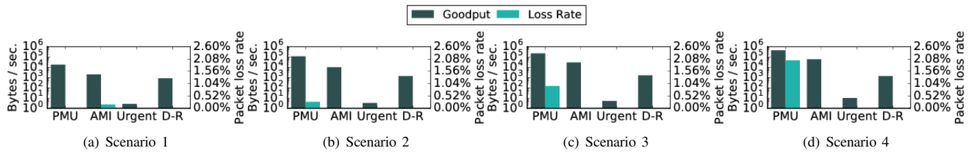
Fig. 4: Goodput rates (left axis) and loss rates (right axis), for each type of traffic. Though the loss rate increases with transmission rate, it remains below 2% in all cases.
